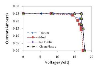
Fig. 7 *I-V* characteristics for irradiation of 255 W/m<sup>2</sup>
