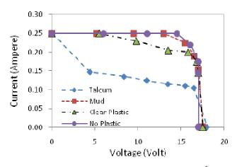
Fig. 9 *I-V* characteristics for irradiation of  $340 \text{ W/m}^2$
