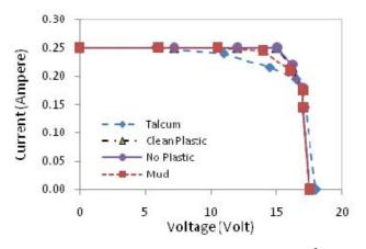
Fig. 8 *I-V* characteristics for irradiation of  $301 \text{ W/m}^2$
