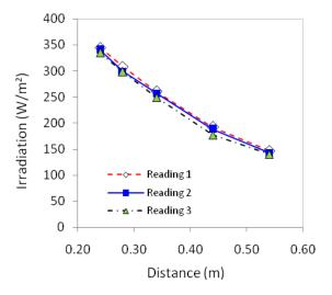
Fig. 6 Irradiation versus distance for two spotlights
