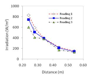
Fig. 5 Irradiation versus distance for one spotlight
